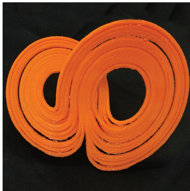
Figure 3. The Lorenz chaotic attractor in equation (4), modeled in Mathematica and 3D printed in FDM PLA.
