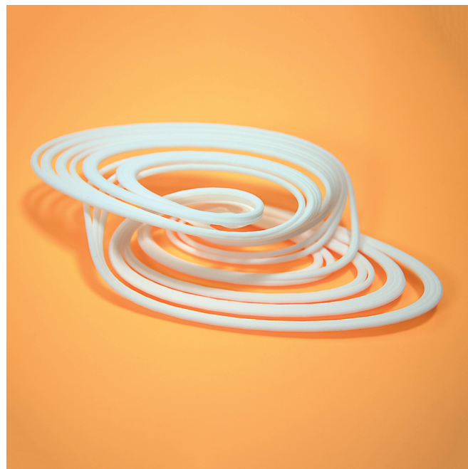
Figure 10. The Arneodo chaotic attractor in equation (7), modeled using the mixed curvature method in Matlab and OpenSCAD, and 3D printed in SLS nylon.
