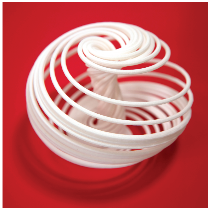
Figure 21. The Langford chaotic attractor (8). Modeled in Matlab and OpenSCAD and 3D printed in SLS nylon.
