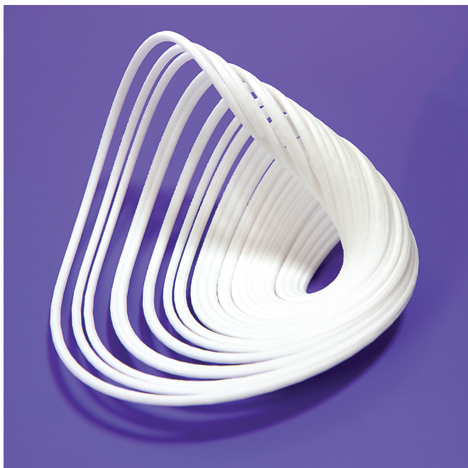
Figure 5. The Anishchenko chaotic attractor in equation (11), modeled in Matlab and OpenSCAD and 3D printed in SLS nylon.
