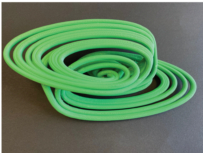
Figure 9. The Arneodo chaotic attractor in equation (7), modeled using the straightforward method in Mathematica and 3D printed in FDM PLA.
