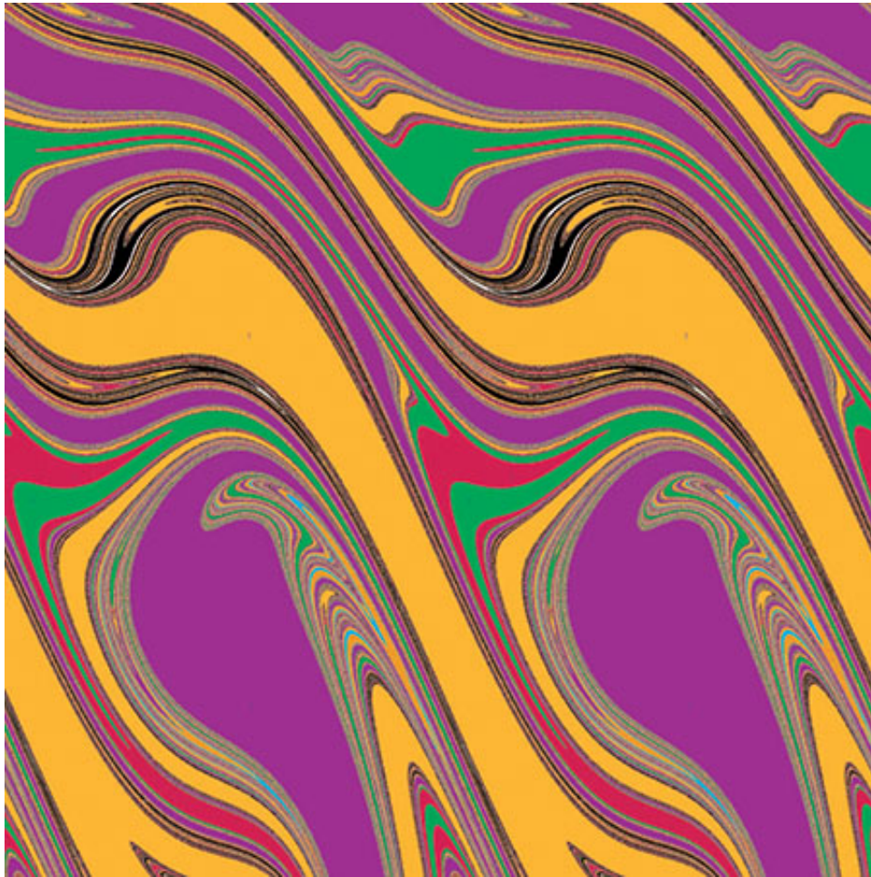
Figure 2. Eight basins of attraction for the forced–damped pendulum. The geometric complexity of the basins results from the chaos on their boundaries.
